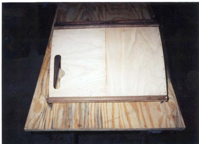
Machine bonnet assembly after adding veneer layer
